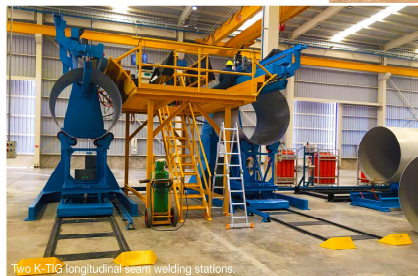
Two K-TIG longitudinal seam welding stations.
