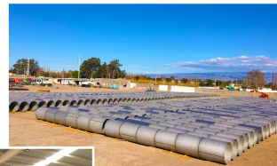
K-TIG welded water pipes awaiting pickup.
